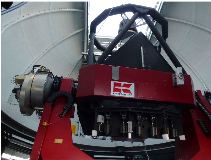
Figure 2.6: WWFI (left) mounted at one Nasmyth port of the Fraunhofer Telescope .
