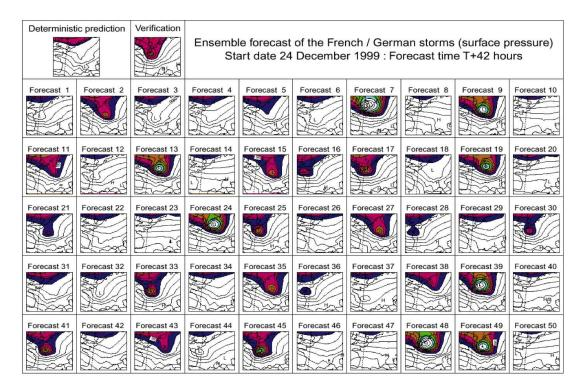
Figure 1.3: Ensemble Forecast of a Storm with 50 ECMWF Model Runs [1, p. 431]
