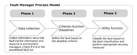
Figure 4.7: Process Model of Fault Manager
