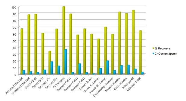
Figure 4: Scavenger treatment to evaluate recovery and chromium levels prior to chromatography.
