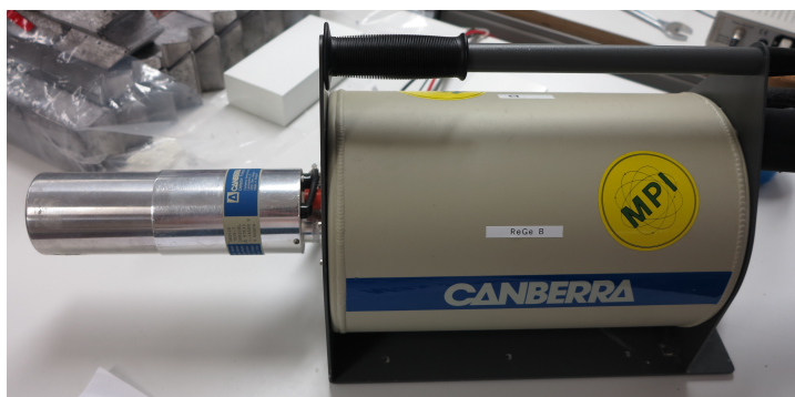
Figure 3.4: REGe detector with the aluminium cryostat on the left and the LN 2 reservoir on the right.
