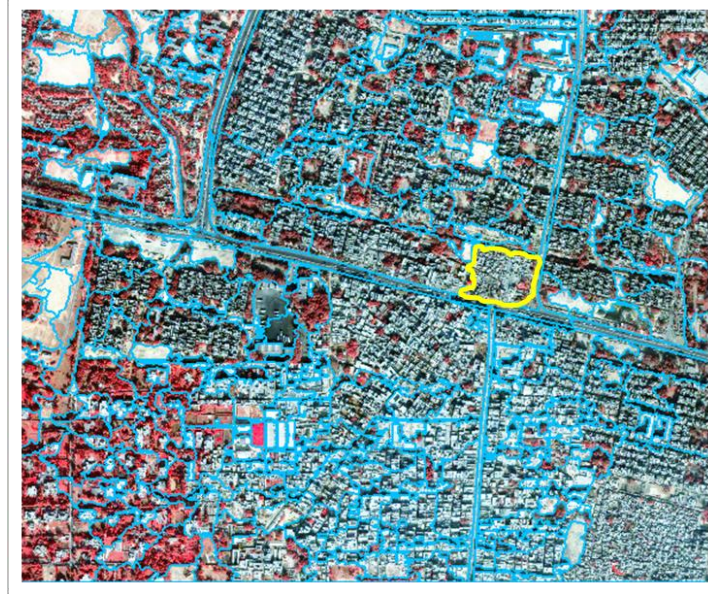
Figure 7-4: Result of multi-resolution image segmentation based on the transfer site South s2: segmentation level 9 with scale parameter 125. The yellow highlighted object delimits clearly the area with the highest building density within this test site. The delineation is consistent with the settlement boundaries of the merging informal settlement areas of Banjara and Harijan Camp .
