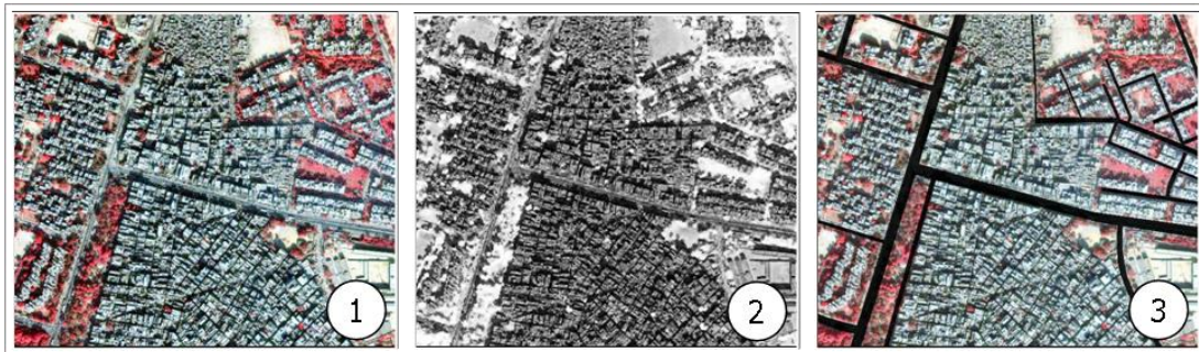
Figure 6-6: Raw data for multi-resolution image segmentation: 1 — training area test site South s3 (channels 4, 3, 2), 2 — NDVI image, and 3 — street layer (manually generated).
