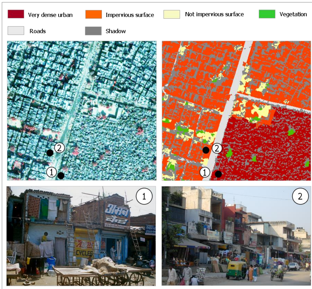
Figure 7-15: Qualitative validation of the classification results using photographs taken during the field campaign 2005 (subset of test site South s3): 1 — Jhuggi Jhompri cluster Nehru and Navjeeewan Camp (informal settlement); 2 — Harijan Colony (upper lower class to lower middle class) (Photographs: S. Smollich, October 2005).
