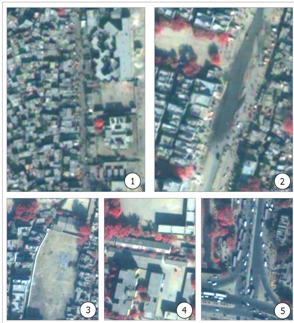
Figure 3-3: Examples for factors that limit the application of pixel-by-pixel classifications of urban environment: 1 — difficult spectral differentiation (spectral similarity of urban buildings and adjacent roads), 2 & 3 — spectral variability (urban road network characterized by different materials alternating within single roads, open space with different or mixed materials), 4 & 5 — phenomena and objects hampering image analysis (shadows of buildings and trees or cars on roads) (Data source: QuickBird test site South s3 and South s2 (4, 3, 2)).
