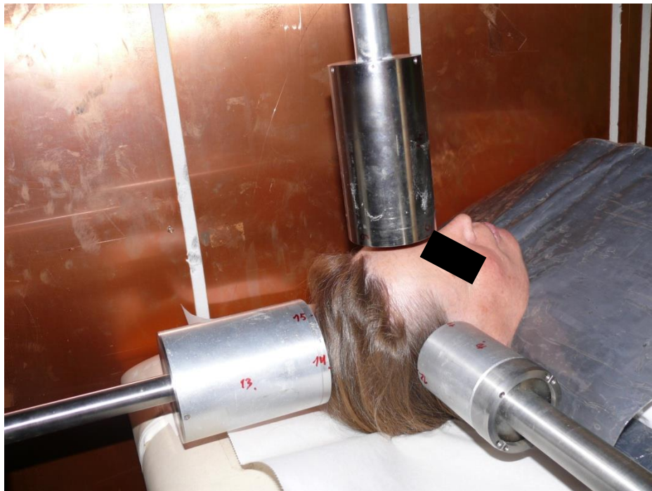
Figure 7.5: Case 2 first measurement at HMGU PBC using a three detectors configuration. On the left detector 4, on the right detector 3, and on the top detector 6.
