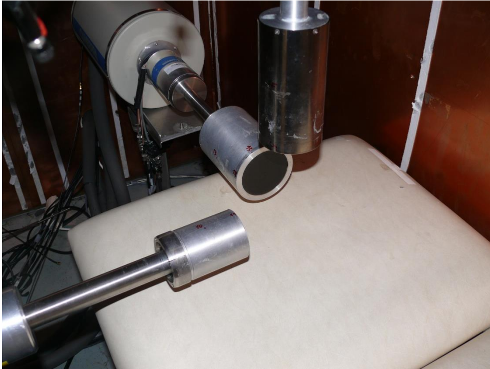
Figure 7.2: HMGU PBC three detectors configuration used in the first measurement including an adjustable medical bed. On the left detector 3, in the middle detector 4, and on the top detector 6.
