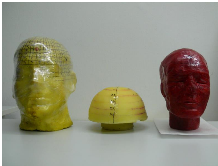
Figure 2.6: Head phantoms used for the HMGU PBC calibration: USTUR case 102 phantom, CSR phantom and BfS phantom, from left to right.
