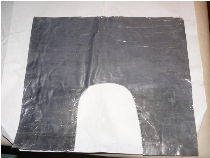
Figure 7.1: Lead shielding designed and constructed to shield the body from the skull; it is made of 5 mm thick lead foil and covered with isolation tape to prevent lead poisoning.
