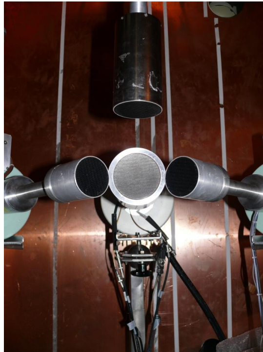
Figure 2.1: Partial body counter germanium detectors in skull measurement geometry configuration, on the right detector 2, on the left detector 3, in the middle detector 4, on the top detector 6.
