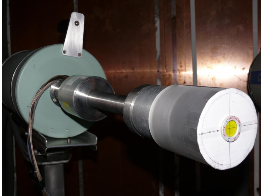
Figure 4.3: Detector 3 and ^{241}\text{Am} point source in irradiation geometry at 5 cm distance.
