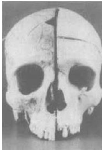
Figure 2.3: Construction of USTUR case 102 skull phantom, on the left case 102 half skull on the right non-contaminated half skull (Hickman and Cohen 1988).
