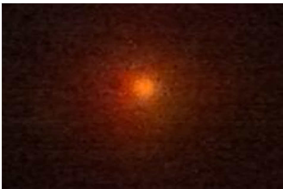
Figure 9.2: Photography of the TPEF signal of rhodamine 6G in methanol. This photography shows the orange fluorescence signal of the fluorophore after multi-photon excitation with intense 1064 nm light.
