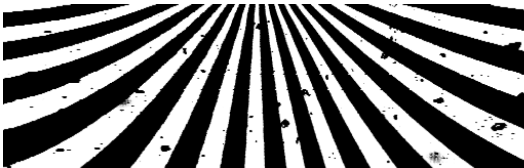
Figure 8.2: Image of a Siemens star acquired with slower speed at the translational stages. This slower speed prevents the “wavy” washout due to the velocity ripples of the stages (cf. Figure 8.1).
