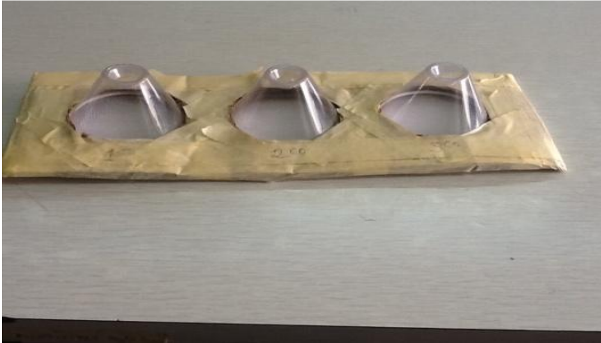
Figure 4.6.1.1: WHO cone fixed on insecticide treated netting to determine the residual activity of the formulated insecticide on the net
