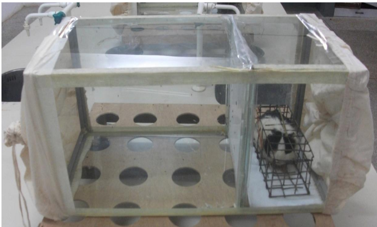
Figure 4.6.2.1: Glass tunnel use in tunnel bioassay to evaluate insecticide treated net in the laboratory
