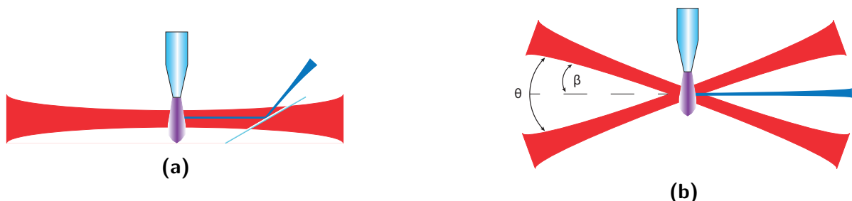
Figure 4.1: Sketch of generic high harmonic generation geometries: (a) collinear HHG, (b) non-collinear HHG
