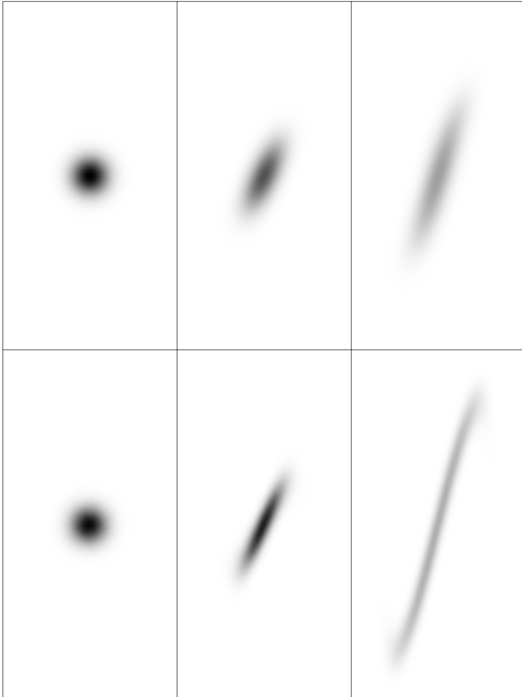
Figure 4.14: Phase space (x,p) evolution of the quantum mechanical Husimi function starting from an instability (top row). Classical Liouville evolution of the same initial function. (bottom row)
