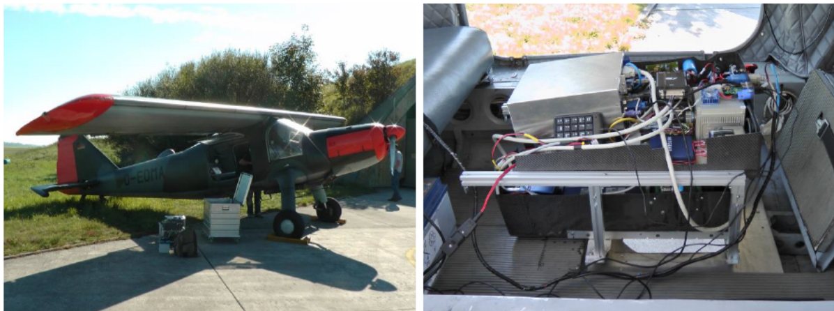
Figure 2-13: Aircraft Dornier Do 27 (left), and AVIS-3 attached above the bottom flap (right).
