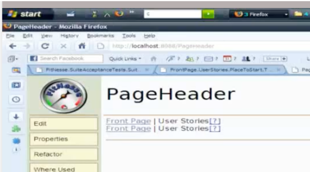
Figure 8.5: Errors aren't always evident. The wiki syntax entered to link to "User Stories" resulted in a to-be-created marker when rendered on the HTML page. This is indicated in the figure with a question mark.
