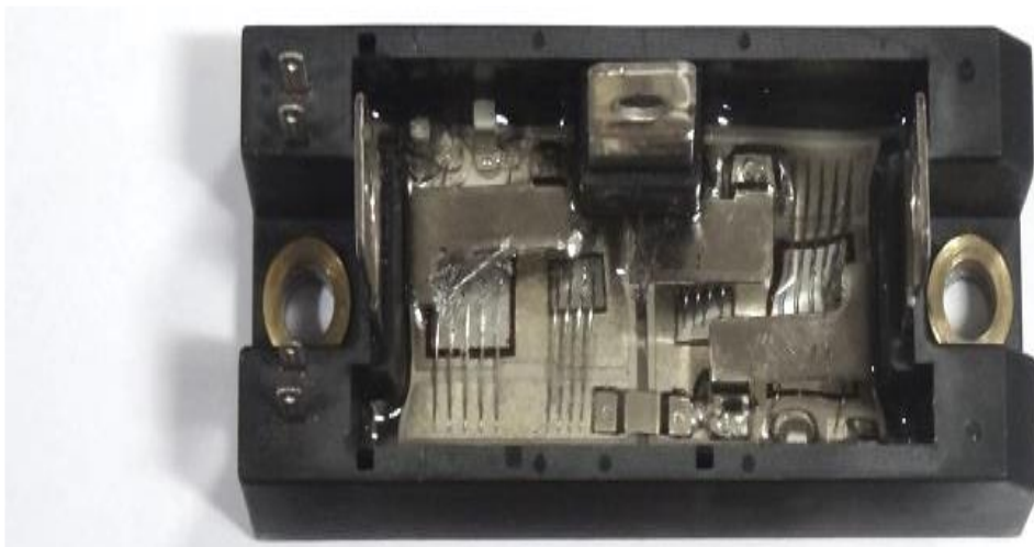
Figure 6.2: 1.2 kV/150 A Fairchild half-bridge Power Module implemented in a silicon IGBT and PiN diode for each switching cell.
