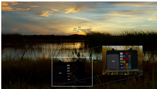
Figure 1: Captured with an ARRI Alexa camera and tone mapped for print; 10.6 f-stops of dynamic range in a sunset scene with a minimum lighting level of 2.8 \text{ }^2 and a maximum of 4,400\text{cm}/\text{m}^2 . Note detail is lost in the tone mapping process. Image courtesy of Brian Karr.
