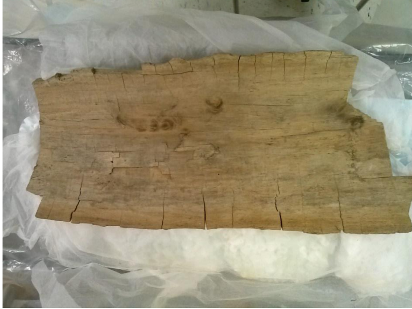
Figure 5: Image of Canoe 3 (PHL0003.001) fragment illustrating the condition of the canoe before retreatment.
