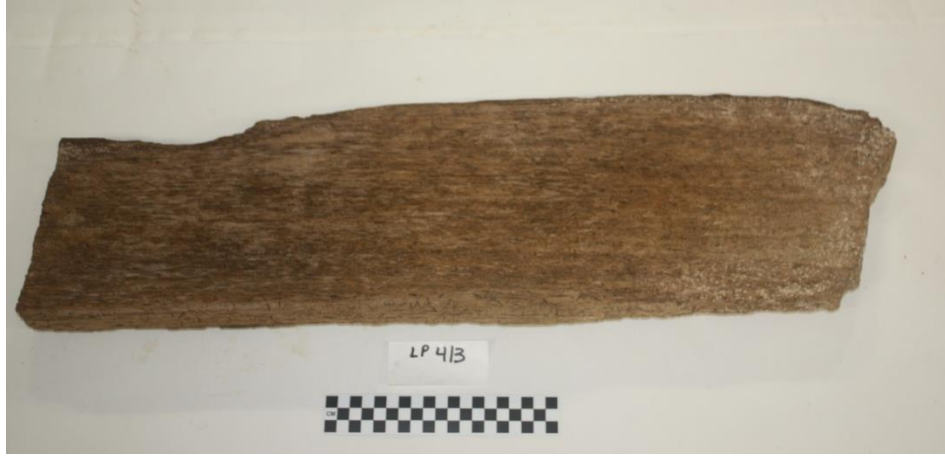
Figure 37: After misting treatment experiment of PHL0004.003, after five treatments.
