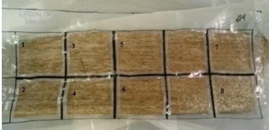
Figure 24: Canoe fragment PHL0004.003 example illustrating the use of a Mylar stencil and location of specific samples; 1 – Control sample; 2 – 100% RO water with cotton swabs; 3 – Hand tools; 4 – 100% etoh solution with cotton swabs; 5 – Dry brushing; 6 – Soot sponge; 7 – Kimwipes tissue poultice with a 100% etoh solution; 8 – Laponite gel poultice with a 100% etoh solution.
