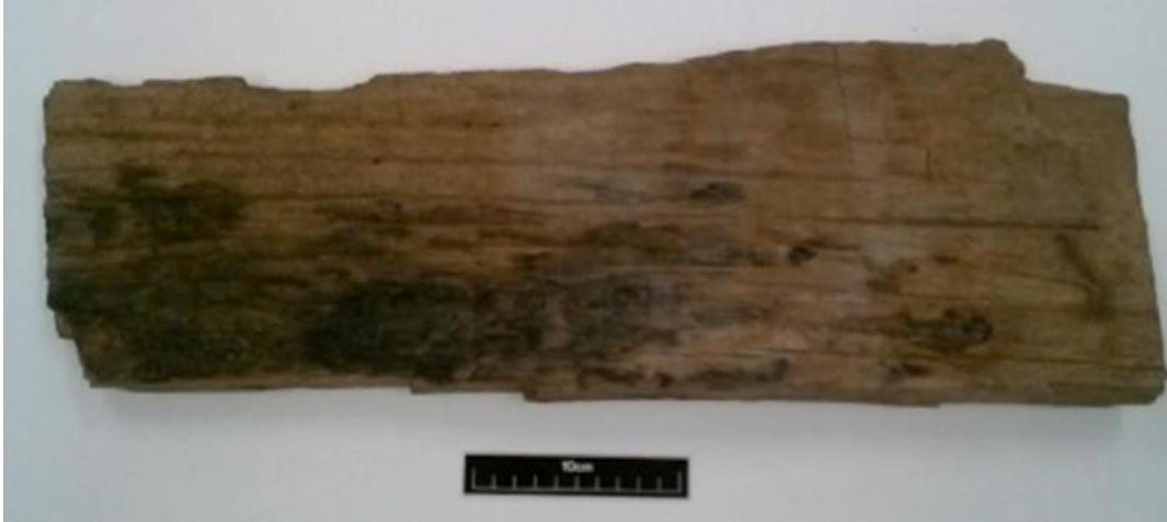
Figure 26: Canoe fragment PHL0003.004 showing after treatment results of the experimental trials.
