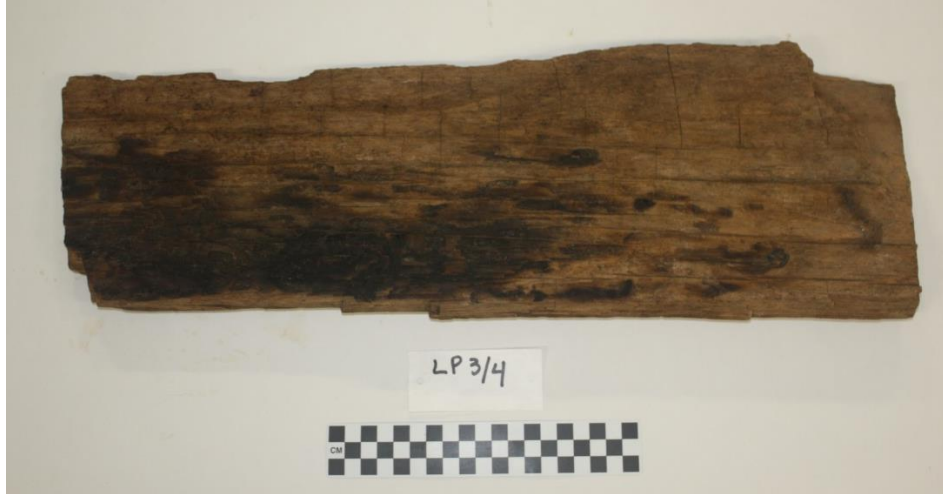
Figure 34: After misting treatment experiment of PHL0003.004, after five treatments.
