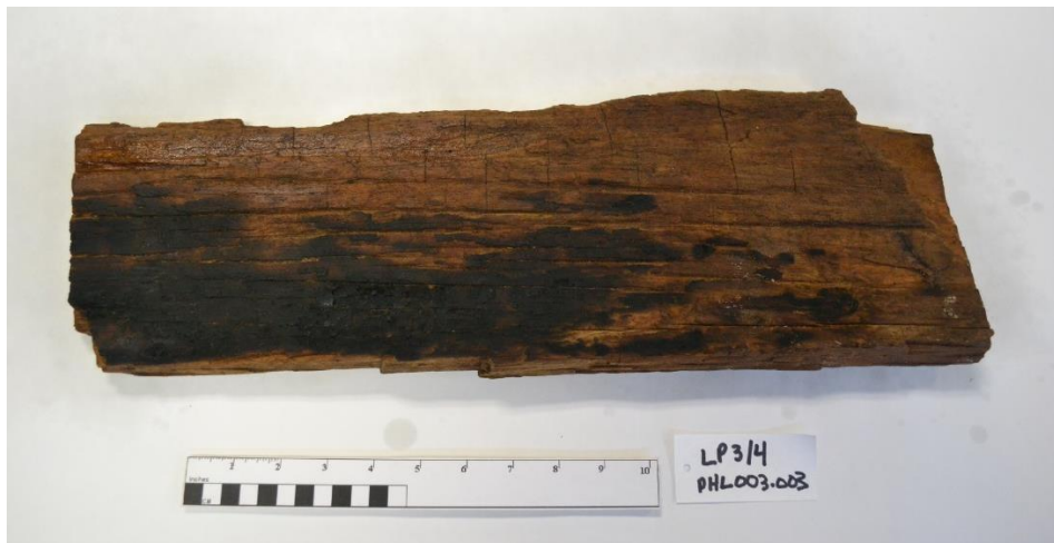
Figure 33: During misting treatment experiment photo of PHL0003.004.
