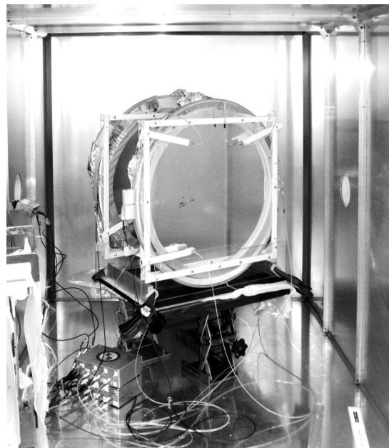
FIG. 5. Dual-drum assembly test article mounted in the hypervelocity impact chamber. Drum diameter is nominally 0.5 m and the impact chamber is a cube with 1.2 m sides.
