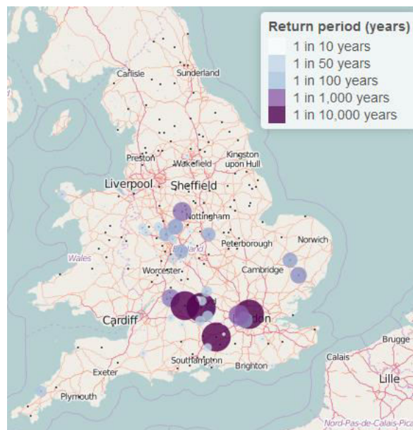
Figure 2. Surface water scenario 1 – high return periods in southern England, with London being particularly affected.
