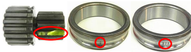
Figure 9.6 Tooth defects simulated on the sun gear and two kinds of inner race defect on deep groove ball bearing
