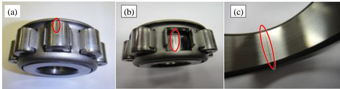
Figure 6.10 Photographs of fault bearings
