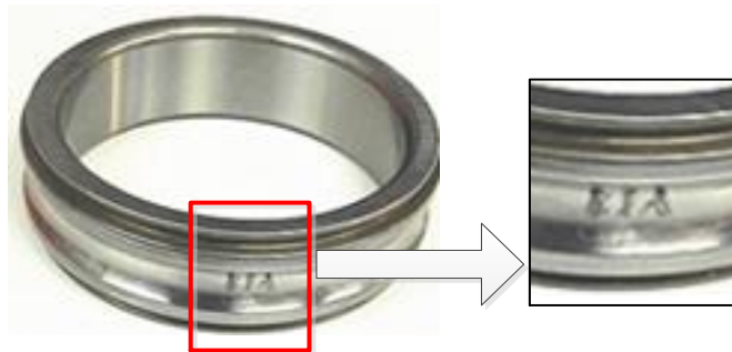
Figure 7.16 Inner race defect on bearing
