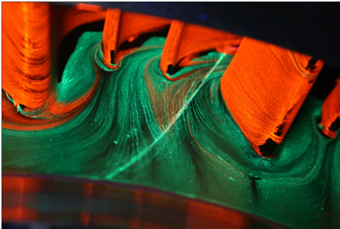
Fig. 10: Flow visualisation on the hub endwall for NGV3(upper) and NGV4(lower)
