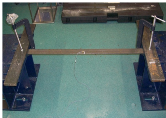
(a) Test beam set-up and attachment of accelerometers
