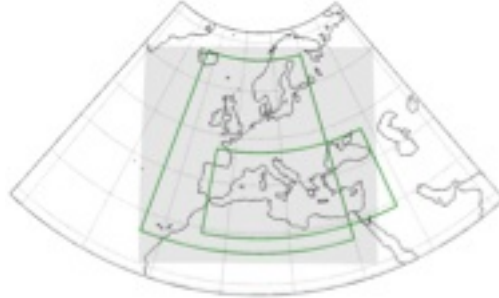
1 2 Fig.7: The gray-shading indicates the SKIRON model domain. The green frames show the areas over which 3 SKIRON passes wind data to the WAM model.
