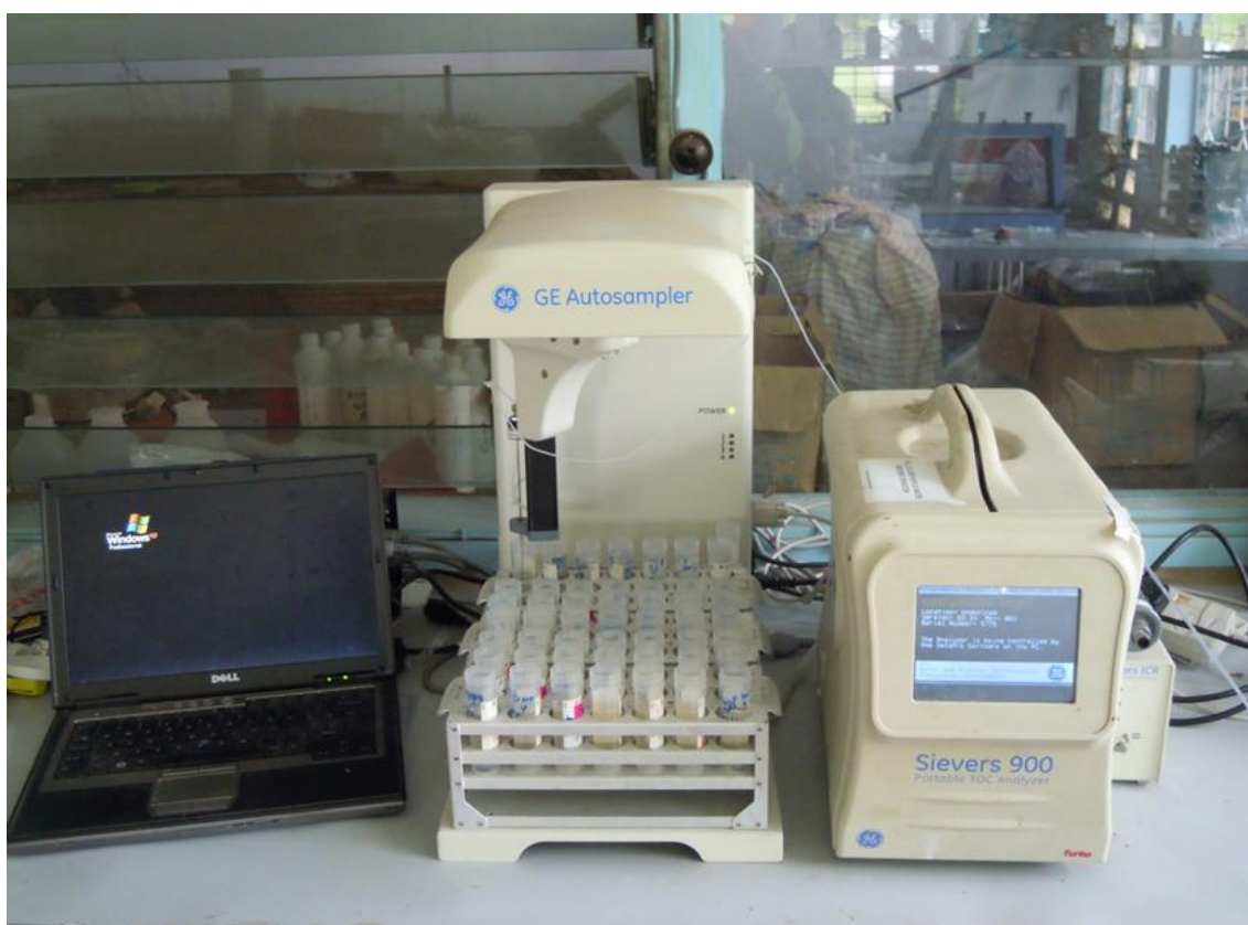
Figure 2.8: Photo of the TOC analyzer with the autosampler on its left side and the ICR unit on its right side
