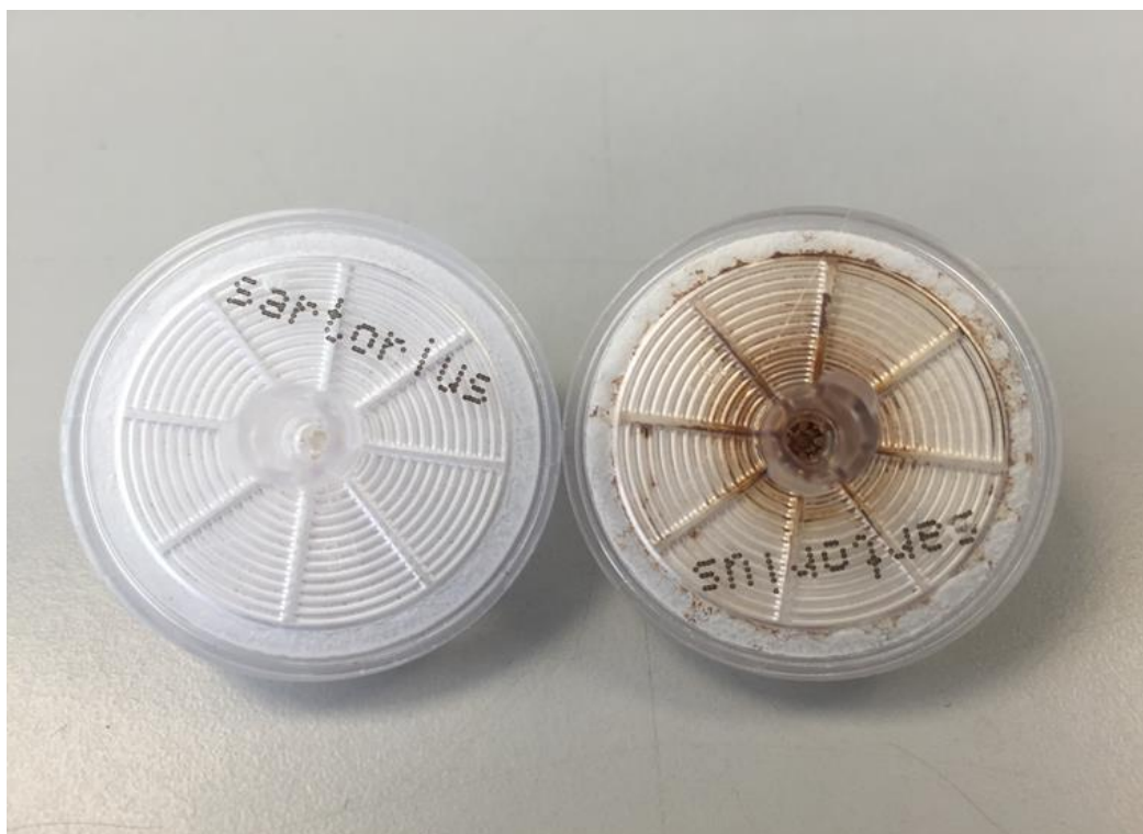
Figure 3.8: Comparison between a new, unused filter and the HS-fouled filter after filtration.
