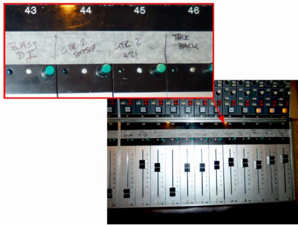
Figure 1. Channel labeling strip on the recording console
