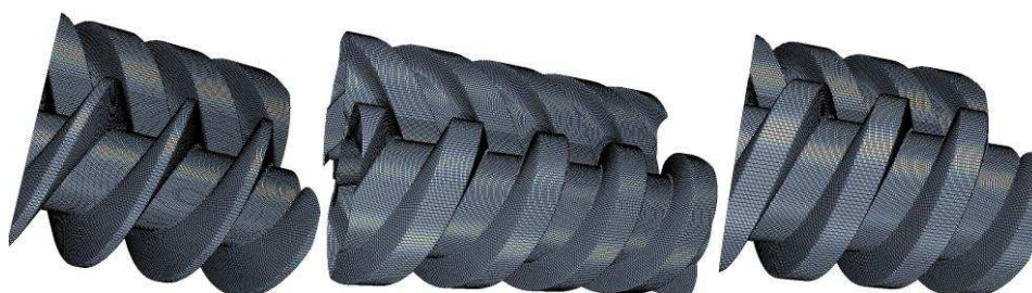
Figure 10 Surface grid of A-type, D1-type and D2-type rotors (from left to right)
