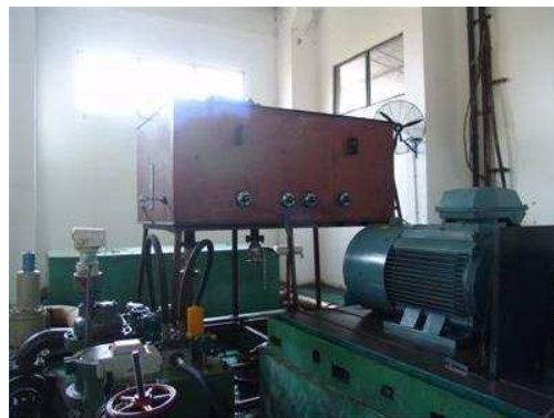
Figure 19 The experimental setup for screw pump performance measurements
