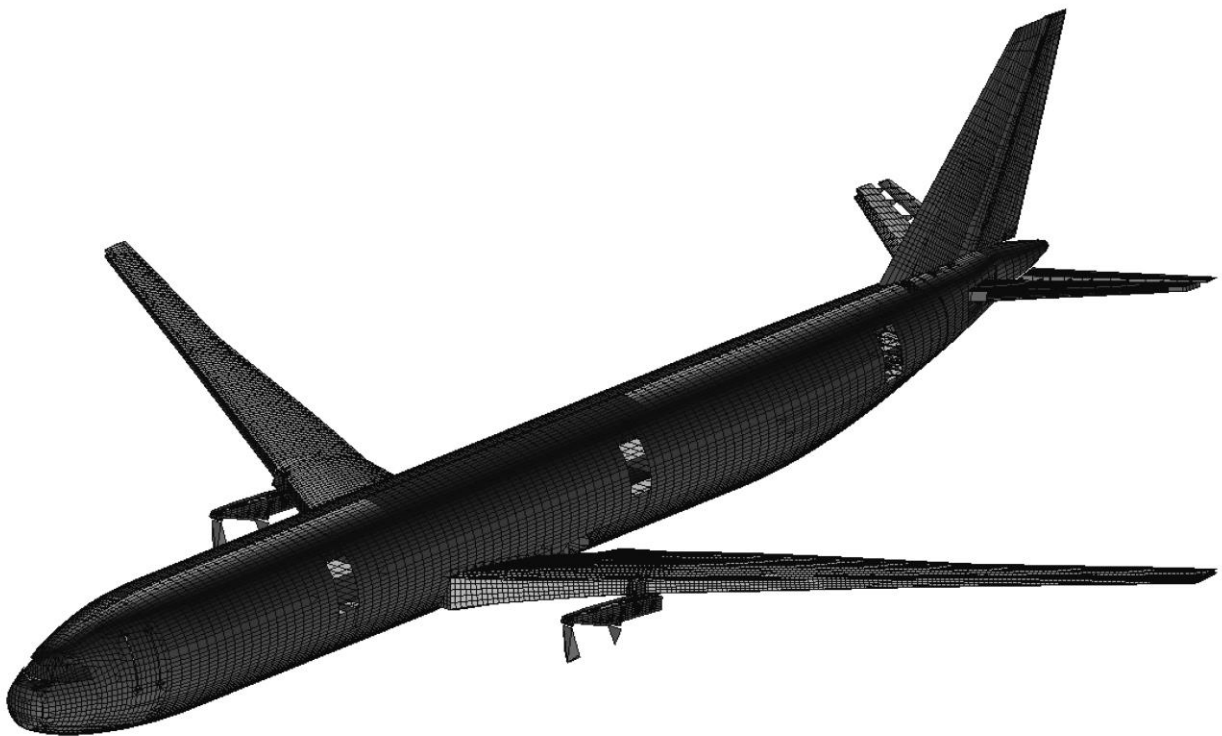
Fig. 10 Industrial standard aircraft GFEM
