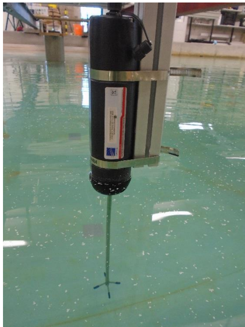
Fig. 4. Photo showing Vectrino Profiler ADV, with model monopile visible in the background.
