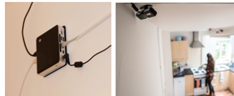
Figure 2. NUC and Asus Xtion sensor in SPHERE house.
