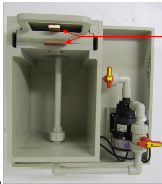
Figure 74: New electrolytic etching machine for the scaled-up process of the Ti sandwich structure, a) side view of the machine; b) front view of the loaded Ti workpiece to the Ti sandwich structure holder; c) top view of the machine with the indicated electrical connections to the sandwich structure and the electrolyte pump.
