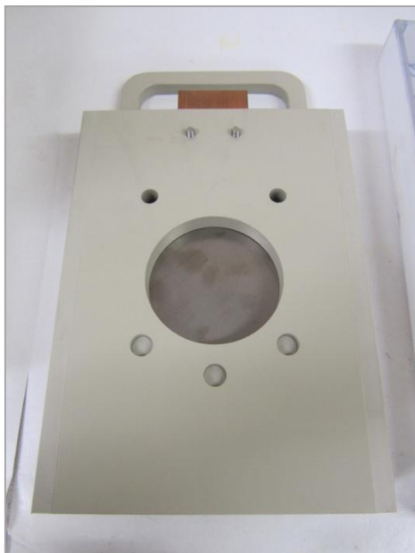
Figure 74: New electrolytic etching machine for the scaled-up process of the Ti sandwich structure, a) side view of the machine; b) front view of the loaded Ti workpiece to the Ti sandwich structure holder; c) top view of the machine with the indicated electrical connections to the sandwich structure and the electrolyte pump.
