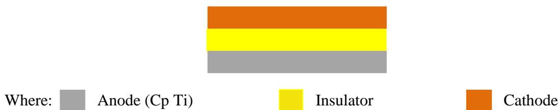
Figure 7: Cross section of the “sandwich structure”.
