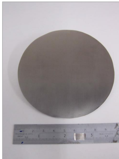
Figure 72: 4 inch diameter manually sanded Ti substrate.
