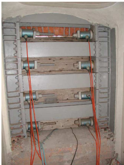
Figure 4. (a) Tie-bar ends equipped with load cells and (b) tie-bars end with the anchorage system.
