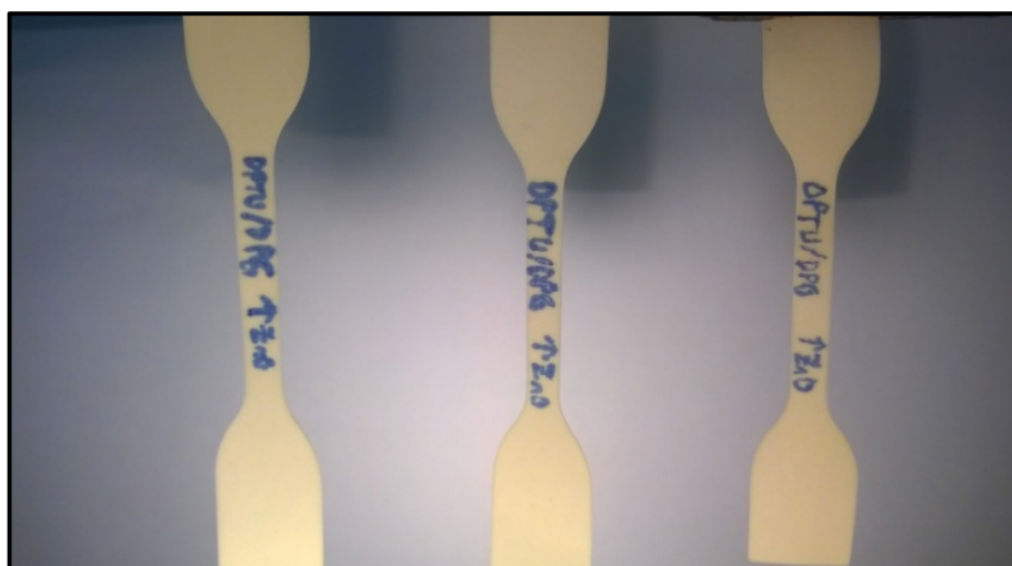
Figure 5.1. Image of the final PCB/DPTU/DPG latex film (A), which has been cut into dumbbells prior to tensile testing.
