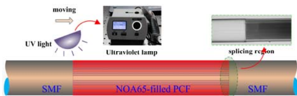
Fig. 2. Schematic of the NOA65-filled PCF. The insets side image shows the fusion joint of the NOA65-filled PCF with a single mode fiber.
