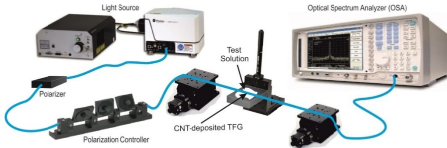
Figure 2: Experimental setup of RI sensing of the CNT-coated 81° -TFG RI sensor
