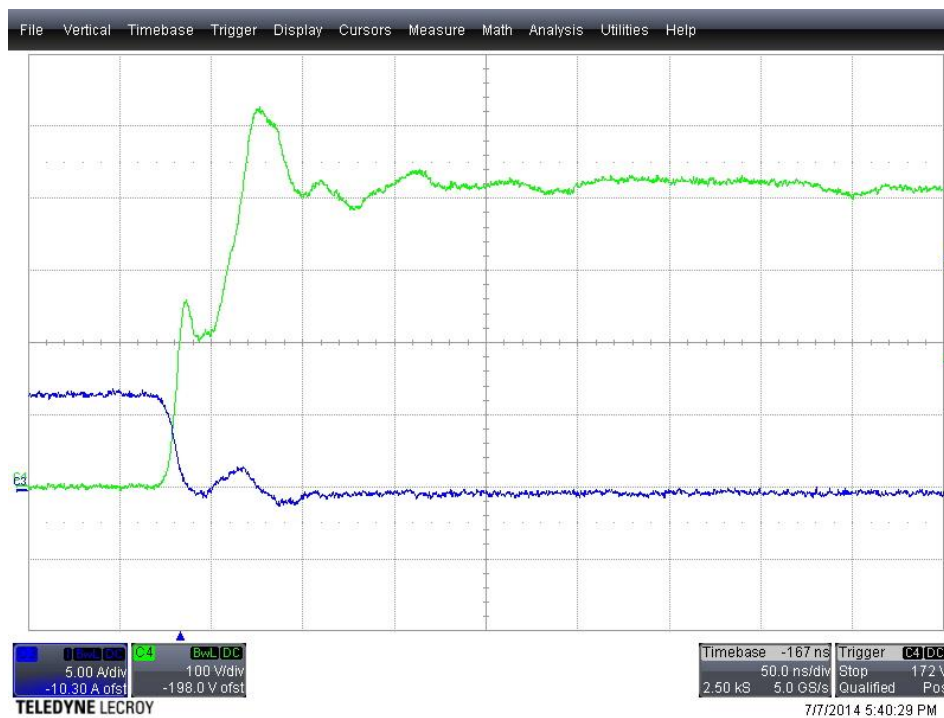
Figure 7.3: Measured waveforms for Q1 turn-off (Voltage 100 V/div, Current 5 A/div, time 50ns/div)
