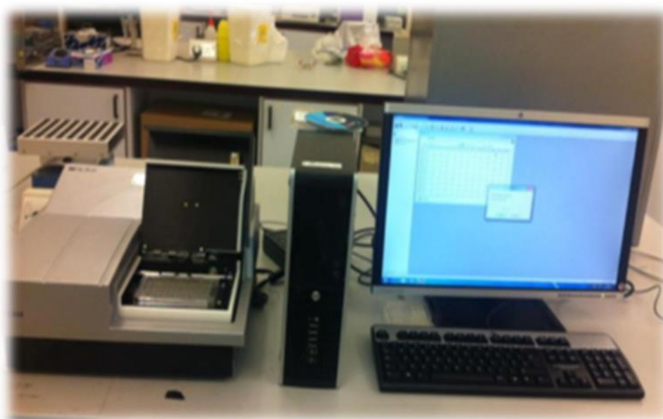
Figure 36 A 96 well micro titre plate placed in the ELx808 absorbance reader, which runs on the Gen5 programme on the PC
