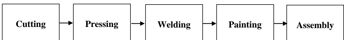
Figure 7.1 Manufacturing process of the lighting sector (Source: author).
