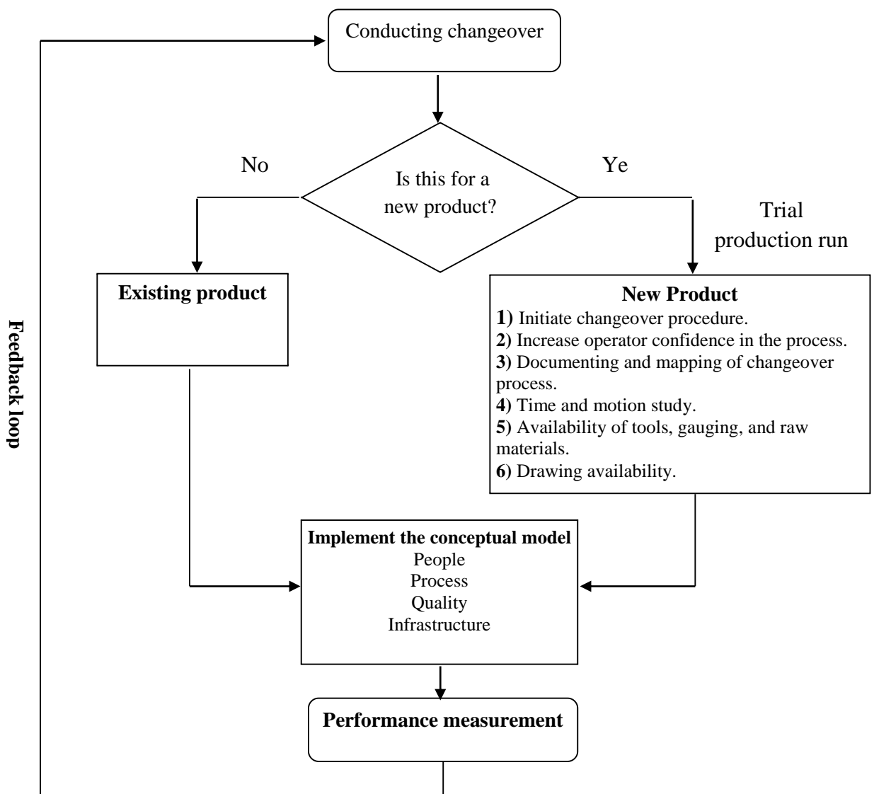
Figure 3. The difference between manufacturing changeovers of new or existing product.
