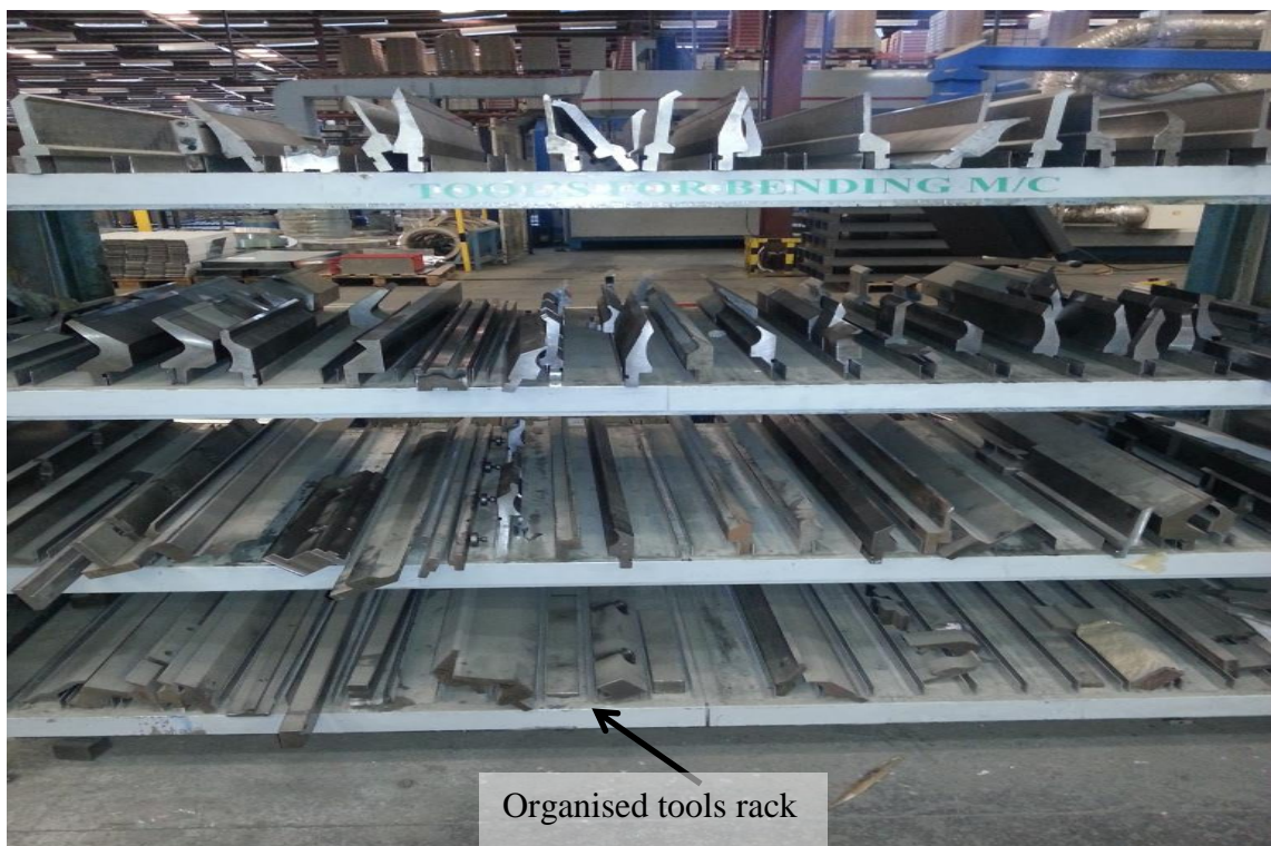
Figure 7.4 Tools rack for bending machines (Source: author).
