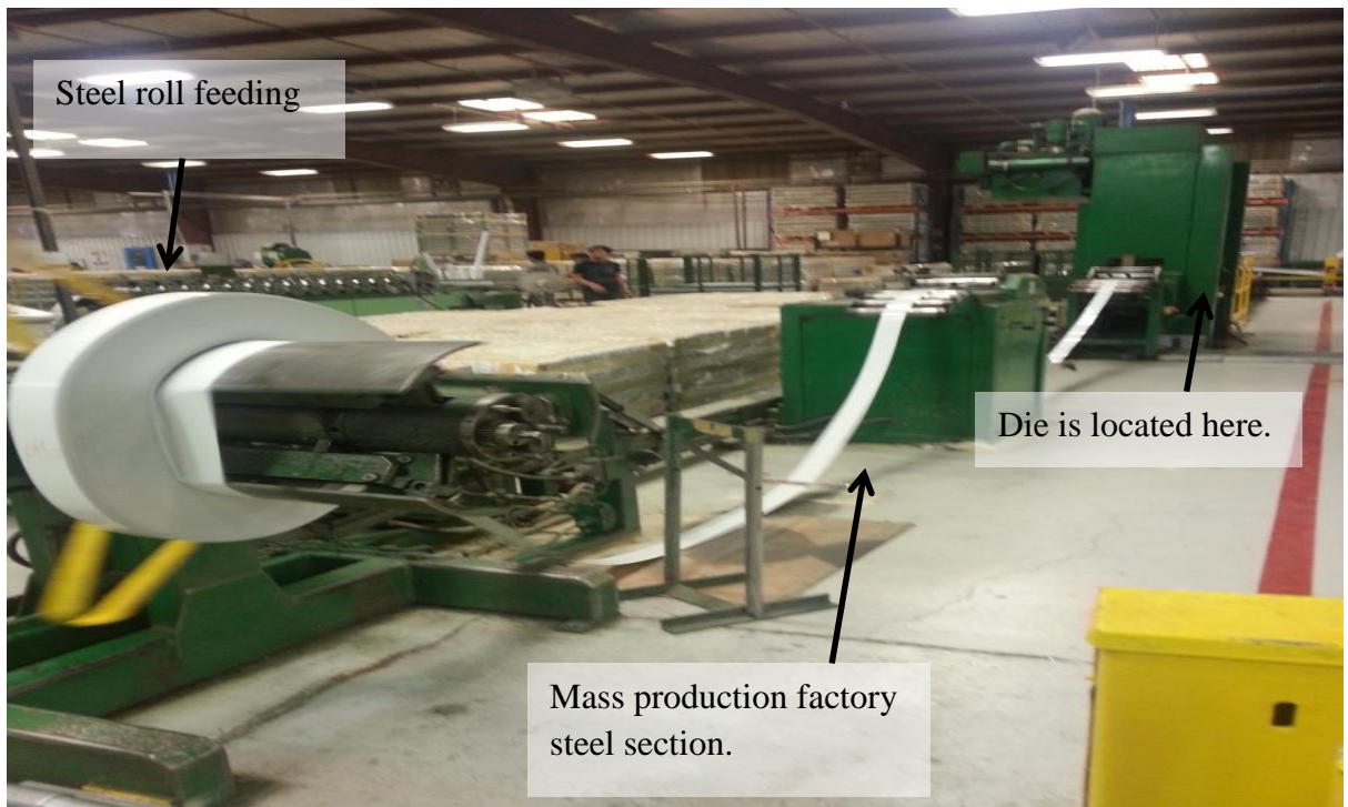
Figure 7.9 Mass Production Factory (MPF) Steel Section (Source: author).
