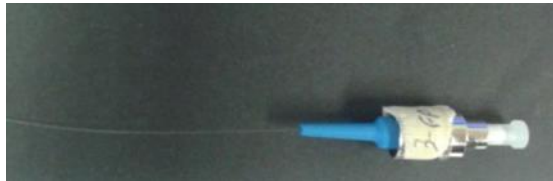
Figure 6. FC-PC connectorised PMMA mPOF fibre
