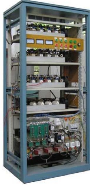
Fig. 8. Prototype of the 6 kW single-phase hybrid-clamped five-level inverter.
