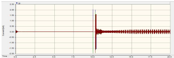
Fig. 6. Simulation results of failure to auto-reclose.
