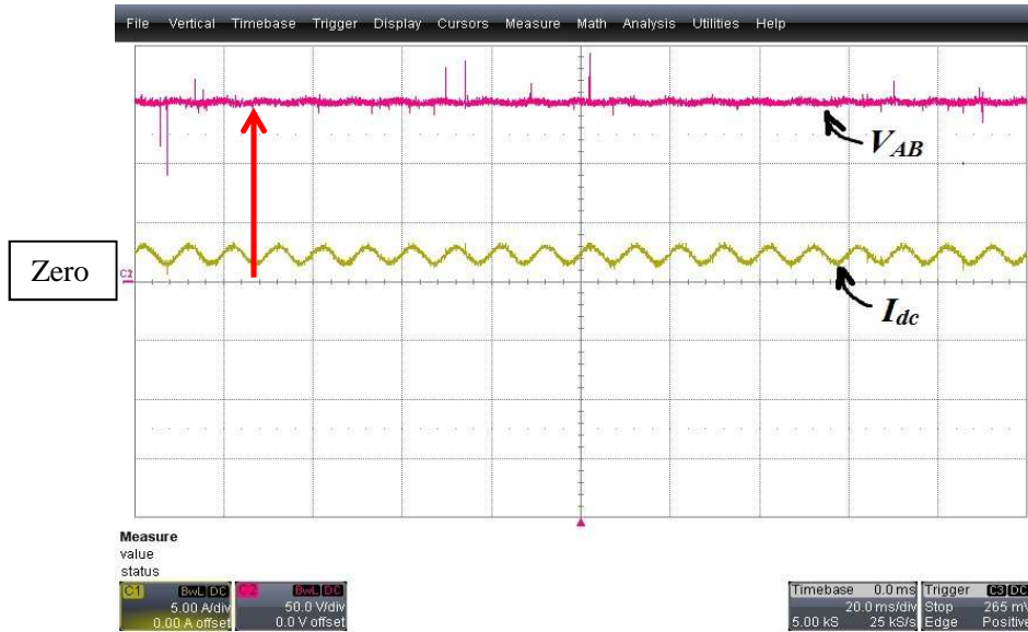
Fig. 3.10 Cascaded boost mode of operation: Experimental result – 2 (time scale 20ms/div, voltage scale 50V/div, current scale 5A/div)
