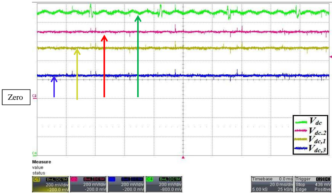
Fig. 3.8 Cascaded boost mode of operation: Experimental result – 1 (time scale 20ms/div, voltage scale 20V/div)
