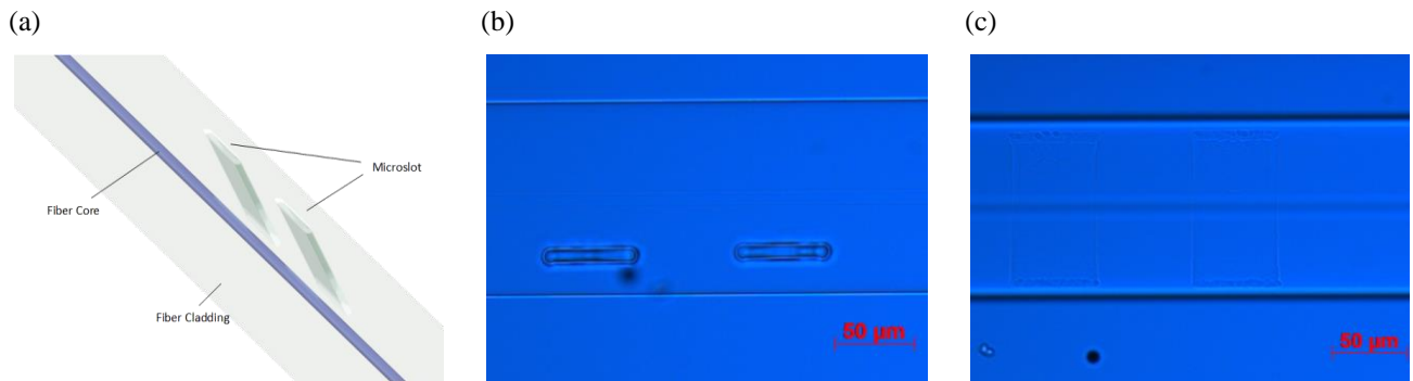
Figure 1. (a) Schematic of the magnetic optical fiber design – femtosecond laser inscribed and etched microslots positioned at the midpoint of the UV inscribed LPG. Image of the in-fiber microslots after femtosecond laser inscription and HF treatment - (b) top view focused at the center of the microslots and (c) side view showing the microslots passing through the whole fiber.
