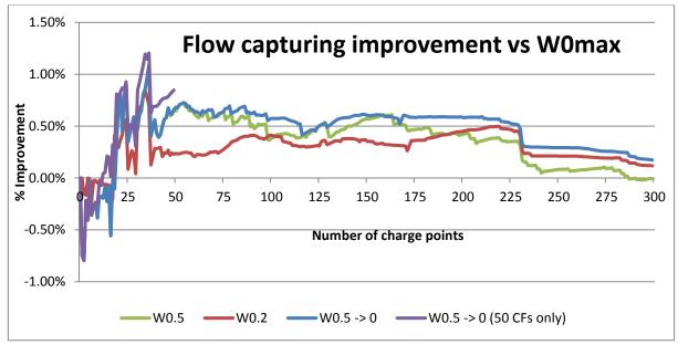
Figure 5-17 - Flow-capturing improvements of weighted heuristics vs W0max
