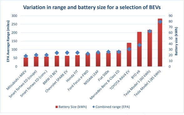
Figure 1-19 - Variation in battery size and vehicle range for a set of BEVs
