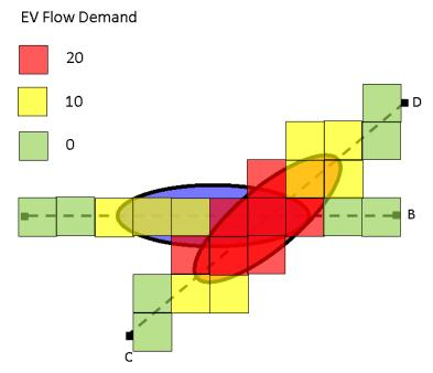
Figure 3-22 - Application of a grid to quantify route flow demand
