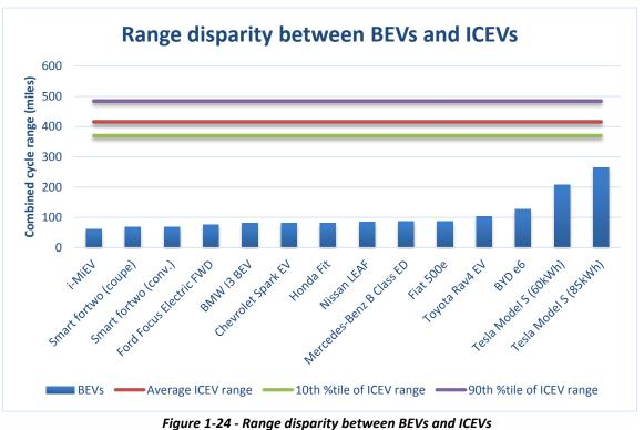
Ure 1-24 - Kange alsparity between BEVS and ICEVS Data Source: (US Department of Energy, 2014) Vehicle ranges calculated from provided combined duty cycle figures (101 ICEV set)
