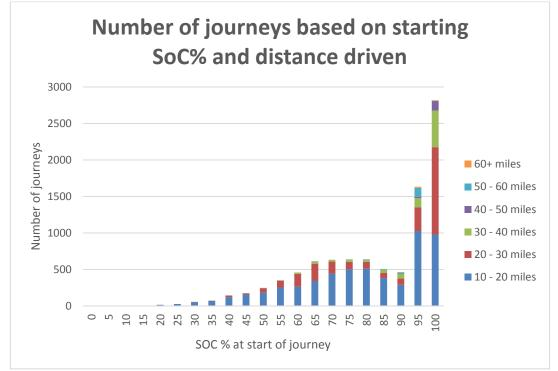
Figure 3-12 - Starting SoC% based on following journey distances Data Source: CABLED trial – see section 1.4
