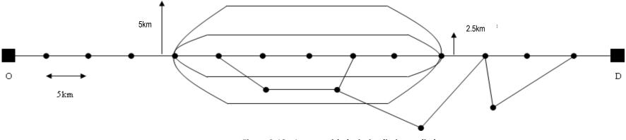
Figure 3-18 - A route with deviation limits applied
