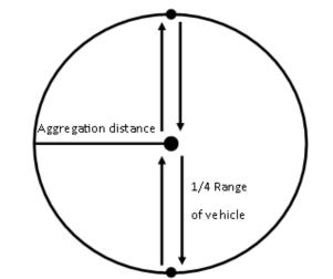
Figure 3-8 - Choosing an aggregation distance to match vehicle range
