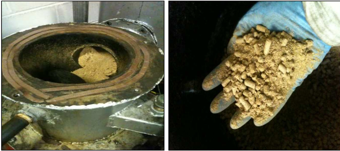
Figure 57 (left) Pellets broken into fines within screw feeder, (right) collected BSG fines and pellets
