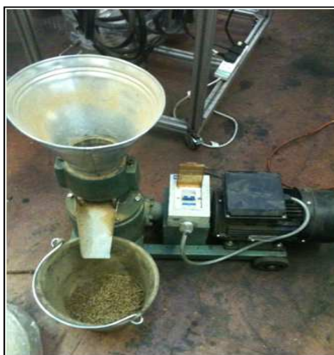
Figure 31 Roller shaft pellet mill with BSG pellets
