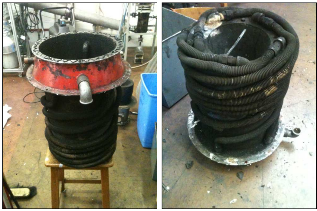
Figure 48 Gasification reactor and pre-heated air inlet pipes
