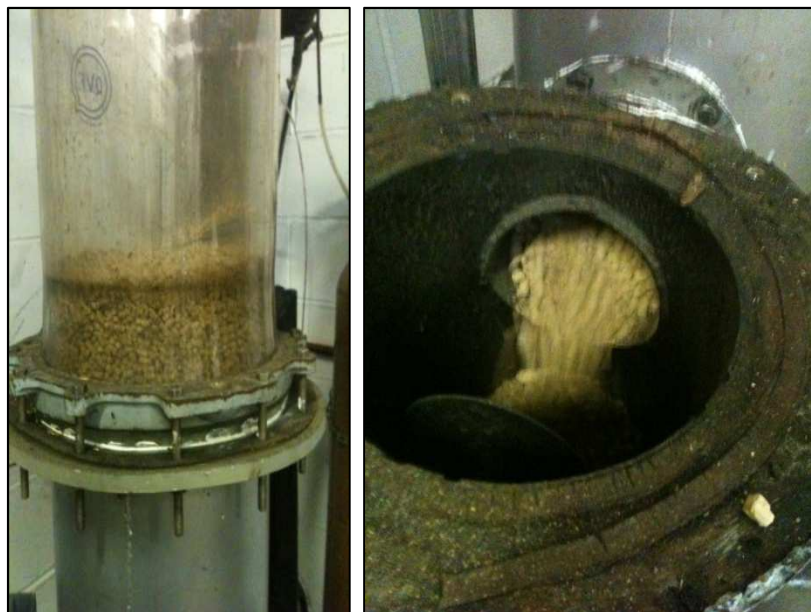
Figure 52 (left) Feed hopper with BSG pellets (right) screw feeder feeding BSG pellets
