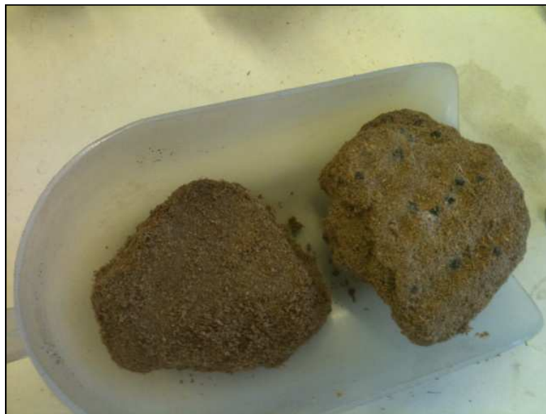
Figure 38 (right) Wet BSG with signs of degradation, (left) dried and ground BSG material
