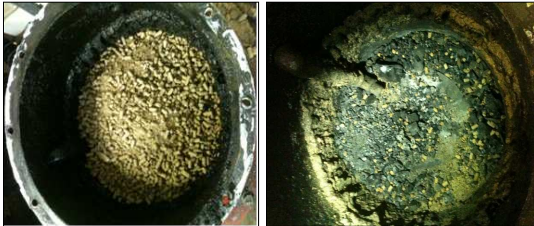
Figure 58 (left) unprocessed pellets and fines (right) BSG ash and char
