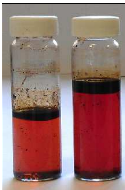
Figure 76 Bio-oil samples received different heating rates (left) 25°C/min (right) 50°C/min
