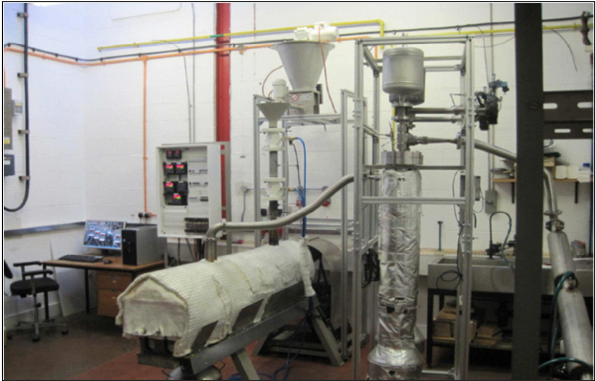
Figure 59 The Pyroformer 20kg/hr. Intermediate pyrolysis unit
