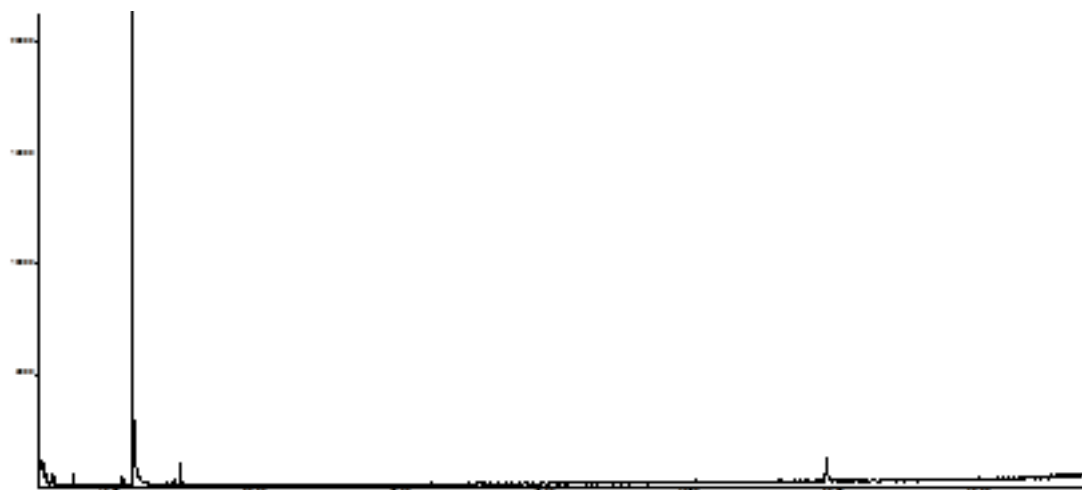
Figure 98 GC/MS analysis of BSG Intermediate pyrolysis oil after catalytic reforming at 850°C with steam (Chemical abundant vs. Retention time)
