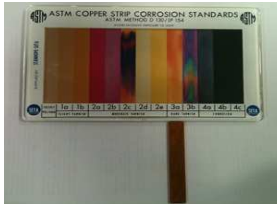
Figure 66 Copper strip immersed in BSG bio-oil after 24h/40°C
