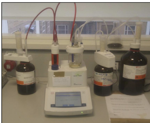
Figure 51 Karl Fischer titration: Water condensate analysis
