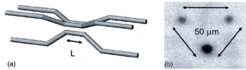
Fig. 1. (a) Schematic of the symmetric three-waveguide directional coupler. Waveguides are initially separated by 50 \mu\text{m} and by 5 \mu\text{m} in interaction region L . (b) Inverse gray-scale CCD image of the waveguide outputs shows a 43:28:29 power-splitting ratio between the guides.
