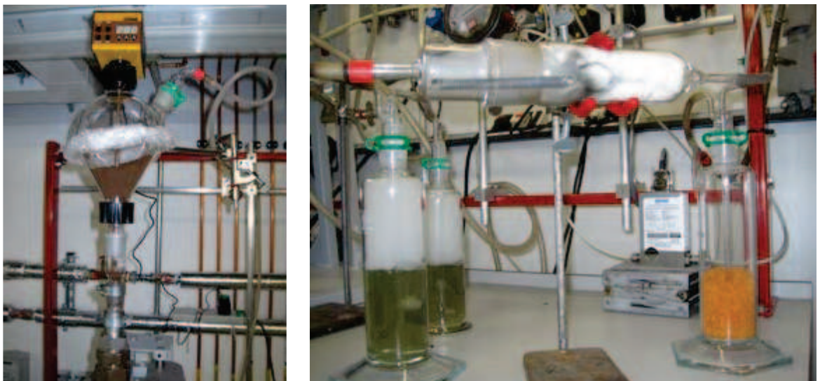
Figure 82. Detailed pictures of the powder dosing feeding system (left) and the liquid collection and gas cleaning systems (right) for the micro-reactor Version 2.
