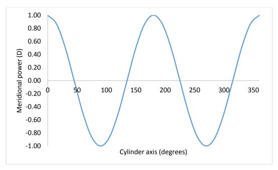
Figure 1.5: Power distribution of a lens with power +1.00DS/-2.00DC x 180.
