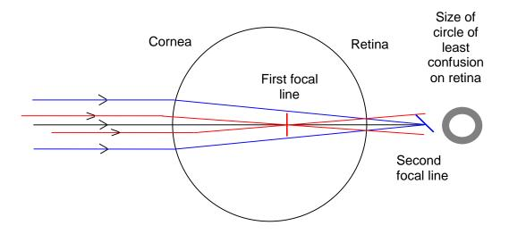
**Figure 1.4:** Light focused in an eye with mixed astigmatism. One line of focus is shown in front of the retina and the other behind it. The circle of least confusion is falling upon the retina in this example.
