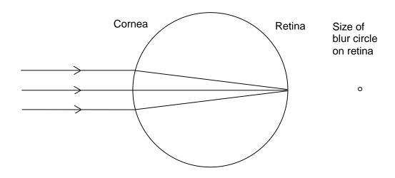
**Figure 1.1:** Light focused within an emmetropic eye. Light is focused upon the retina and the resultant blur circle is very small.
