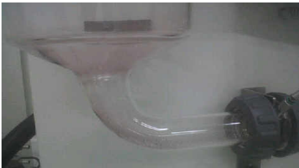
Figure 5.12: Sticking of microparticles at the interior walls of spray dryer. As a result of TPGS tackiness, microparticles sticking occurred on the walls of the instrument leading to degradation of omeprazole (pink colour) and lower process recovery.
