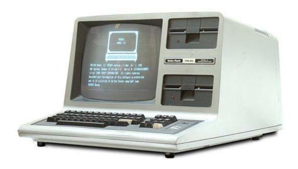
The Tandy TRS-80 was originally introduced in 1977 and used cassette tapes to store data. Sold through Radio Shack stores, the first model racked up sales of 10,000 in the first month at \$600 each. Pictured above is the TRS-80 Model III, which was introduced in 1980 and employed two 8 inch floppy disk drives (touted at the time as a revolutionary breakthrough) – one for the program files and one for storage. There was no hard drive.
