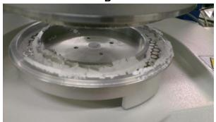
Figure 4.22: Freeze dried mannitol powder adhered to shear cell. A: Shear cell lid with vanes covered with mannitol powder freeze dried from 0.5 M Mannitol at a shelf cooling rate of 5 °C/min. B: sample trough of shear cell expected to hold all powder under analysis.
