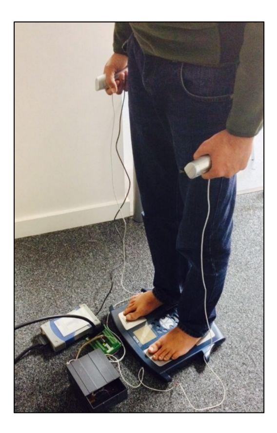
Figure 9-2: Shows a subject undergoing impedance examination on the device (version 4).
