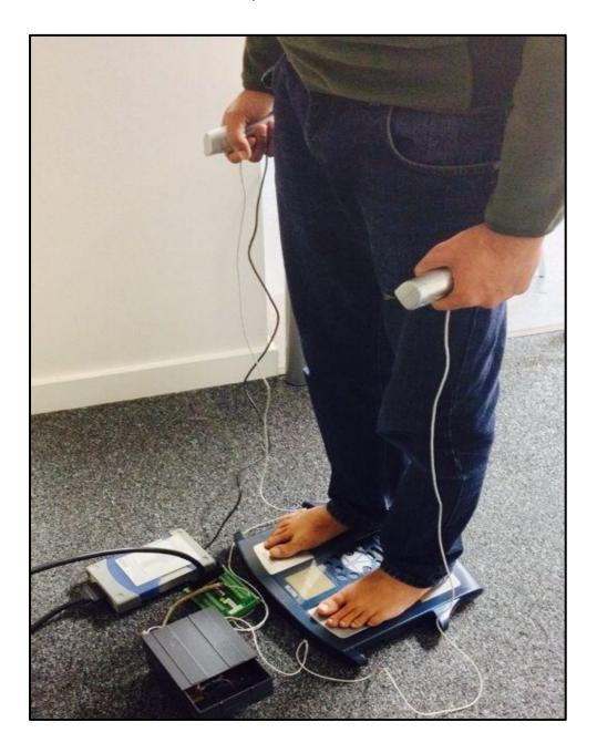
Figure 11-1: Shows a volunteer undergoing bio-impedance examination on device version 4. As stated in section 9.1 the internal circuitry of the Tanita device pictured is replaced with device V4. Table 11-2: Shows the body composition summary from a DEXA. The 'Region' column lists the section of the body and the top row lists the body compositon parameters in grams. Last column represents percentage fat in the particular region.
