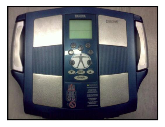
Figure 3-1: Shows the Tanita BC-545 and 8 foot and hand electrodes (two hand electrodes hidden from sight).
