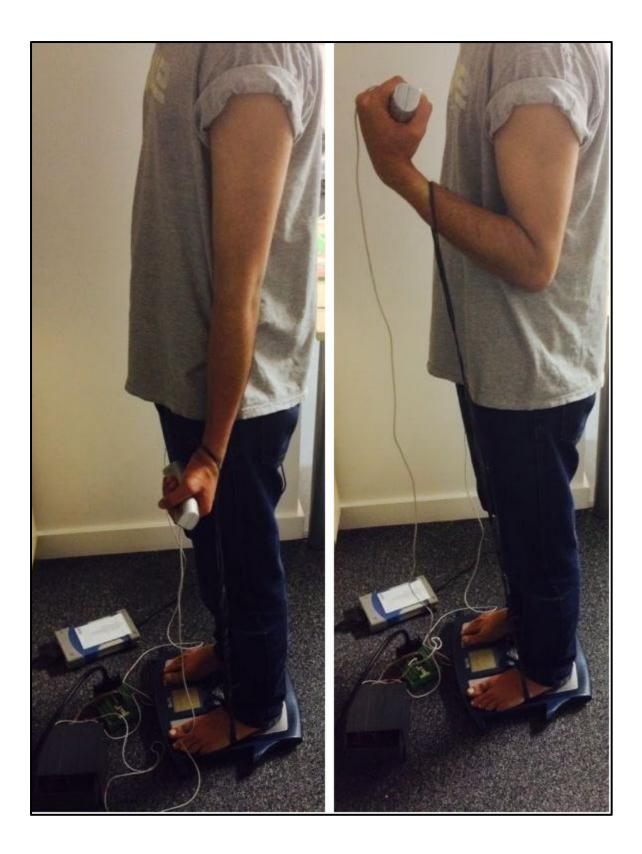
Figure 11-10: Shows the volunteer undergoing impedance measurement while his arm is flexed. Note the elastic band around the wrist and the change in area of cross section of the arm before and after flexing the arm. The procedure utilized V4 of the bio-impedance device and the signals are recorded using Agilent U2531A.
